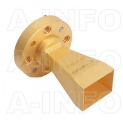
LB-3-25-A Standard Gain Horn Antenna 220-325GHz 25dB Gain Rectangular Waveguide Interface
